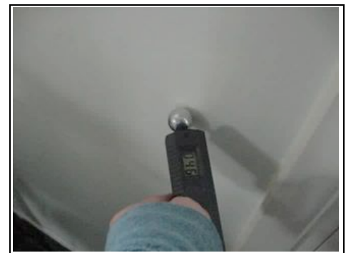
Testing for rising damp
