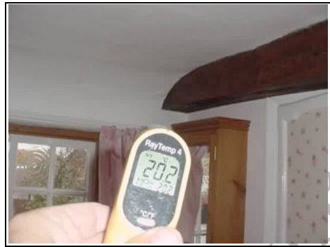
Slightly rounded ceiling in rear bedroom indicates the possibility of cold bridging
