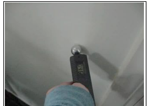
Damp meter reading indicating rising damp
