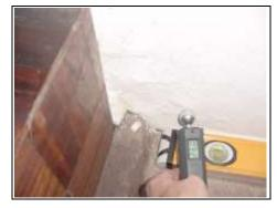
High readings near where staircase has been removed
