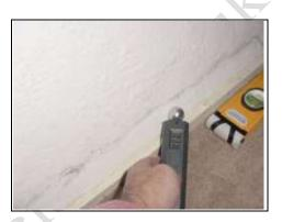
Damp readings taken where the sole plate should be – slightly high
