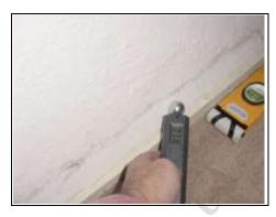
Damp readings taken where the sole plate should be are slightly high
