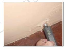
High dampness level noted under the window in the hallway
