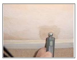
Ground floor testing area of plaster that has come away in hallway-
