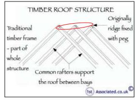
This is what an original timber frame roof would look like. The roof in this property has a ridge board (red)
