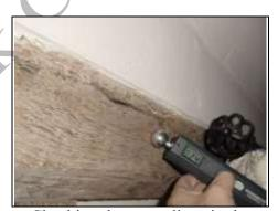
Checking damp readings in the wall plate
