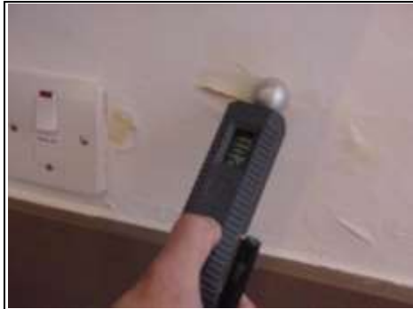
Damp meter readings indicate dampness is coming into the fourth floor via the front parapet wall
