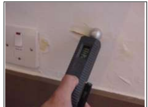
Dampness internally caused by box guttering to front wall
