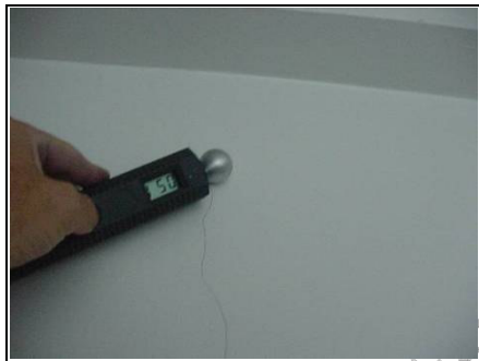
Gann meter readings showing dampness in the WC on the half landing
