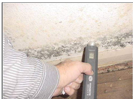
Checking for damp with a Gann meter. Is it rising damp or is it condensation?
