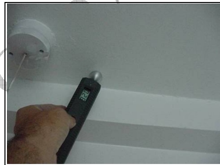
The Gann meter readings showed no dampness on the ceiling
