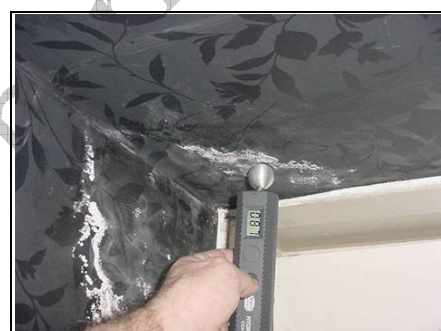
Dampness found using a Gann meter. Is this rising damp or a water leak?
